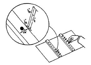
Figure 3. Pin transfer apparatus. The task was to transfer eight pins one at a time from one set of holes to the other. The inset gives the dimensions of pins and holes for the  $W_S = \frac{1}{8}$  in. condition.
